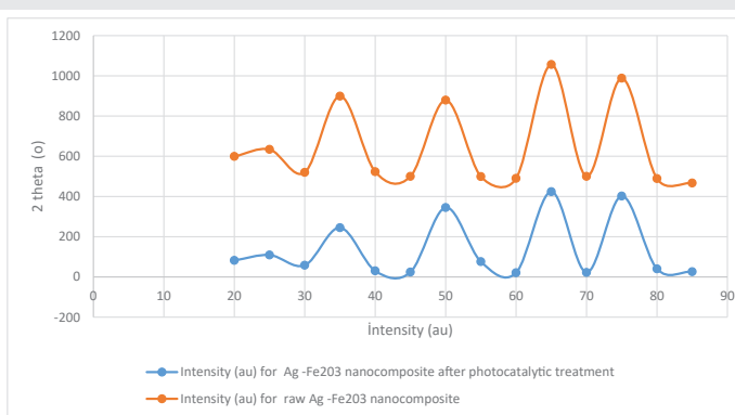
Figure 5: XRD peaks of raw Ag - Fe 3 O 4 nanocomposite before photodegradation and after 20 times photooxidation under sun light for pharmaceutical wastewater containing ibuprofene drug and oxytetracycline antibiotic.
